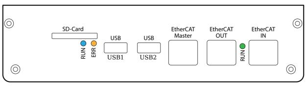
Fig. 4-1 Terminal arrangement on the Q.station 101 (top).
