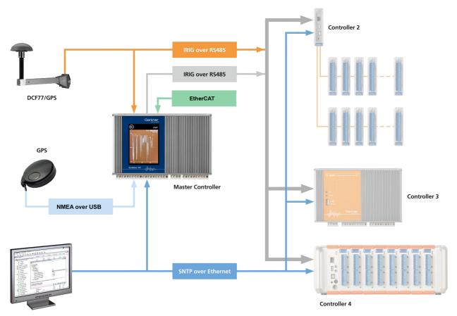
*Fig. 5-3 Possible types of time synchronization.*
