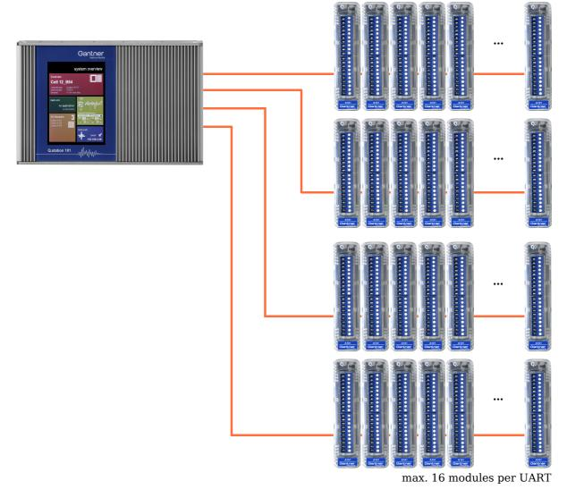
*Fig. 3-1 Q.station 101 with up to 64 modules.*
