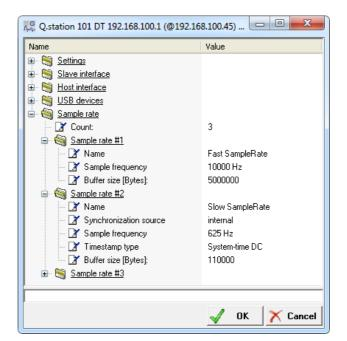
Fig. 7-1 Setting the sample rates
